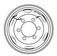
Handhole to handhole. Handhole to studhole. Handhole to rim.
